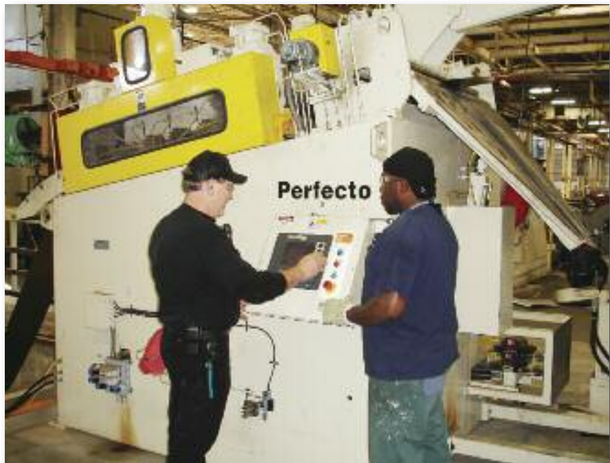
This new feed system provides material to a 1500-ton press at ICE Grenada Stamping & Assembly, Grenada, MS. The line helps produce 4.4 million parts annually for a Tier One customer.
