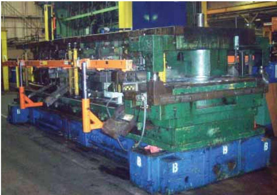
Transfer dies for the 1200-ton press are staged via one of two rolling bolsters, enabling 30 to 45-min. tool changeout between jobs.
