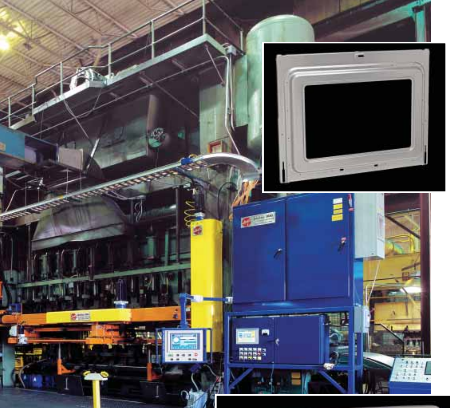
This 1200-ton mechanical press, outfitted with a new three-axis servo transfer system, produces more than 3 million parts per year—in various sizes, draw depths and material thicknesses—at the ICE Acklin Stamping plant. Parts include refrigeration compressor housings, shown at left with other Acklin stamped parts attached, and a stove inner panel and control panel (right).
